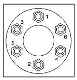
12. Tighten the nuts firmly in a crisscross sequence as shown by turning the wheel wrench clockwise.
